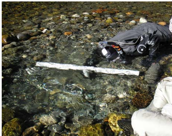
Figure 7. T-shaped PVC device used to ensure bucket placement at depth of 30cm.
