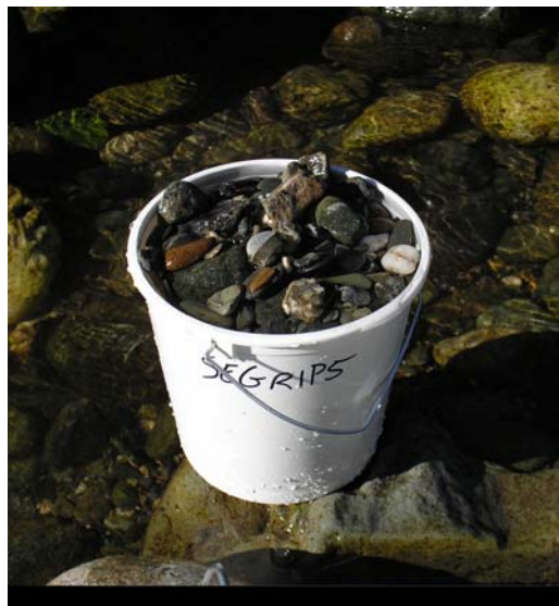
Figure 5. Solid walled, 2.5 liter, PVC bucket were used to monitor sediment intrusion in redds (6 per redd).
